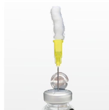
Figure 3. Ventilating T-1 media with a cotton plugged needle. Source: U.S. Centers for Disease Control and Prevention
