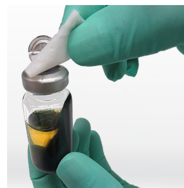
Figure 2. Disinfecting the rubber stopper of the T-1 bottle. Source: U.S. Centers for Disease Control and Prevention
